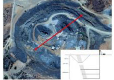
Figure 1: Google earth plan view of open pit and schematic model of crown pillar in OP-UG transition.
